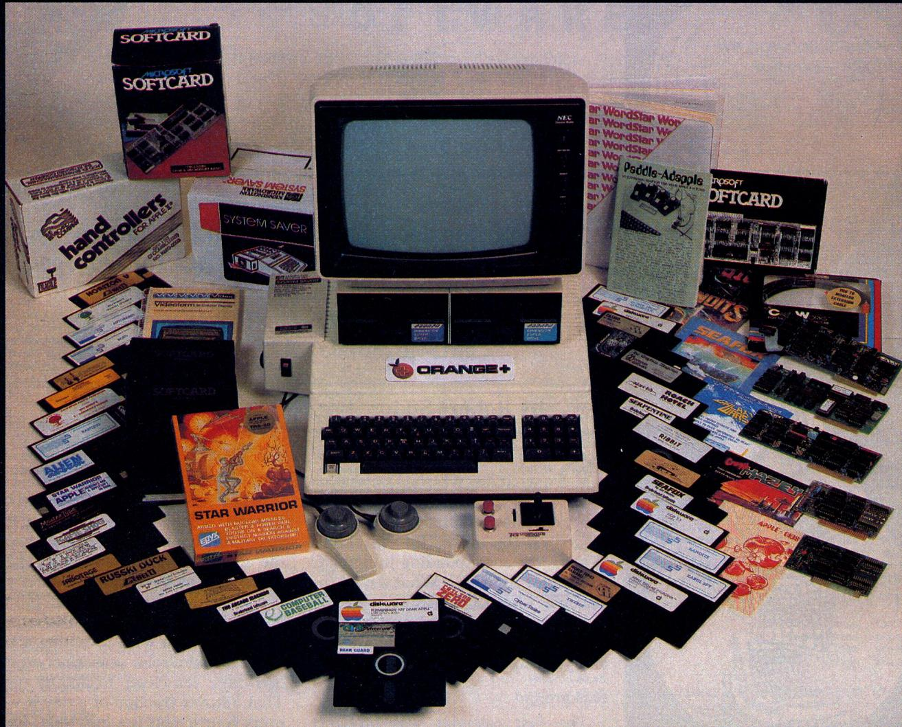
Finally, a dynamic powerful, practical personal computer that is fully Franklin Ace 1000 and Apple® II compatible, yet, lower in price than the competition. Uses existing available software. The "ORANGE+" is the pacesetter of the future, with a **switchable 110-220 volt power supply, upper and lower case with lower case locking key**, enhanced audio and color functions, 8 slot motherboard, game port, fully socketed I.C. board, a 3 ROM operating system, 48K ram, fully expandible.
